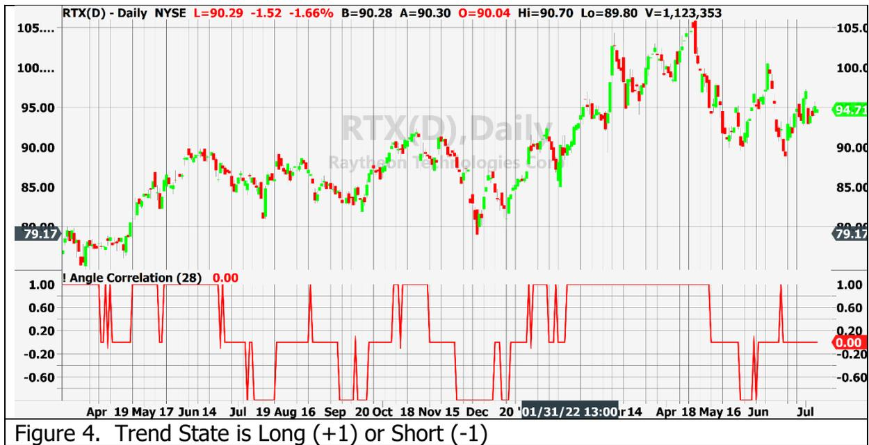
With reference to Code Listing 1, you can replicate the state variable display by removing the curly brackets around the code segment titled "Trend State Variable" and ensuring curly brackets are placed around the other display code segments.
